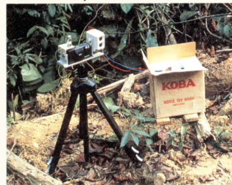
The Olympus*Infinity and infrared beam in the Gbi National Forest, Liberia. Power is supplied by the 12-volt car battery.
